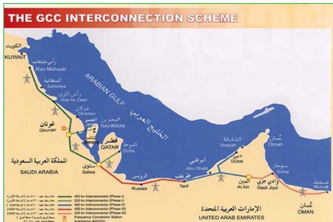
Fig. 39. The interconnection of the GCC regional power grid (GCCIA)
